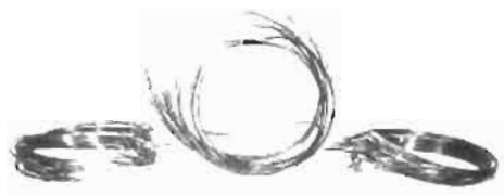
Fig. 3.48. Failure modes of unidirectional rings.
