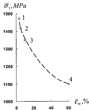
Fig. 4.50. Dependence of the longitudinal strength on the matrix ultimate elongation (numbers on the curve correspond to Figs. 4.48 and 4.49).
