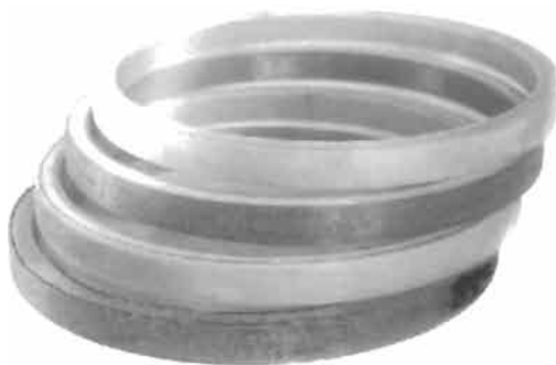
Fig. 5.16. Composite sandwich rings with foam core.
