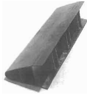
Fig. 4.79. A composite leading edge of an aeroplane wing made of carbon fabric by lay-up method. Courtesy of CRISM.
