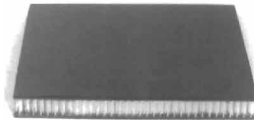
Fig. 5.15. Composite sandwich panel with honeycomb core.
